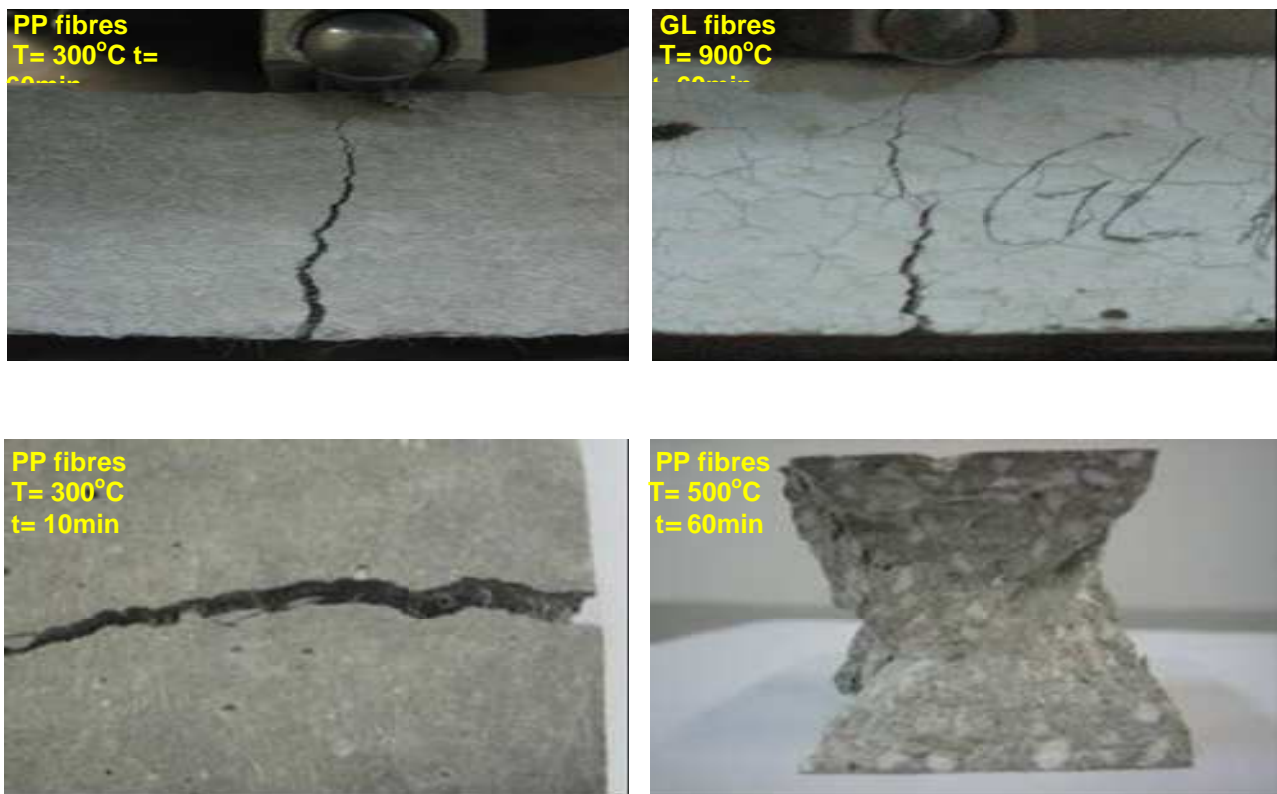
Figure 10: Details of fracture surfaces of specimens after their loading
