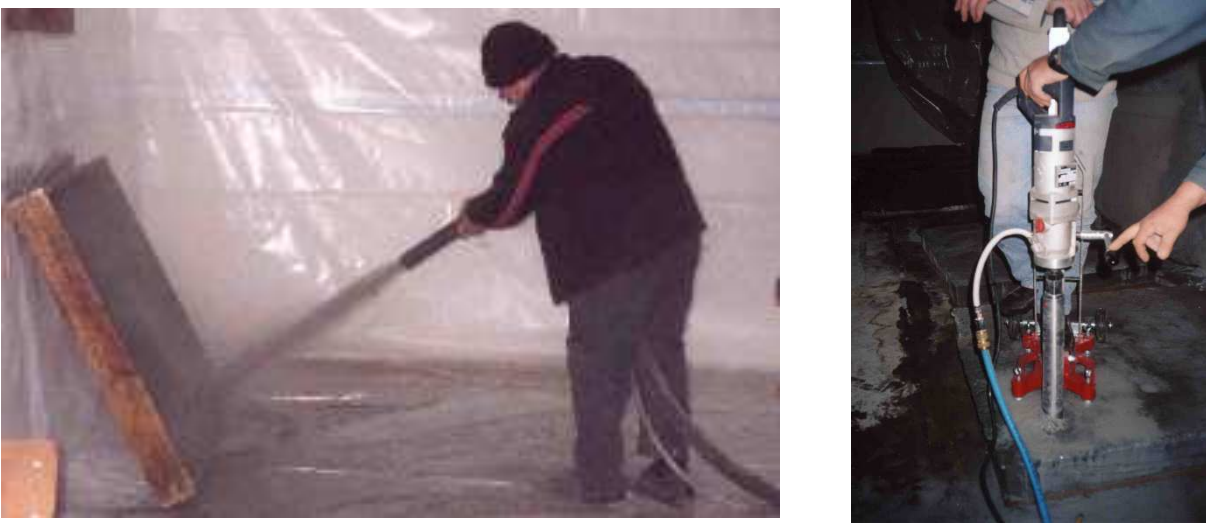
Figure 13: The procedure of spraying mortar into panels under controlled laboratory conditions.
