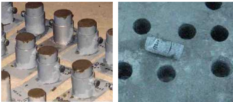
FIGURE 14: Cast specimens into the moulds (left) and cores out off the panels (right)
