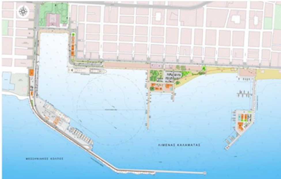
Map 1: Port of kalamata: 1,000m of breakwater, 1,200m of quay walls, 500,000sq.m of port basin
