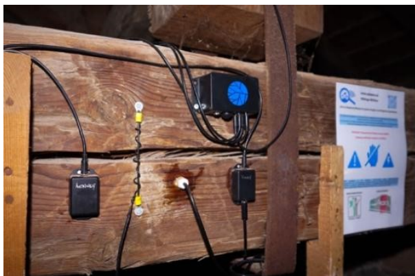
Figure 5. Installation of a “HERMON” device in a 19th-century wooden beam on a roof
