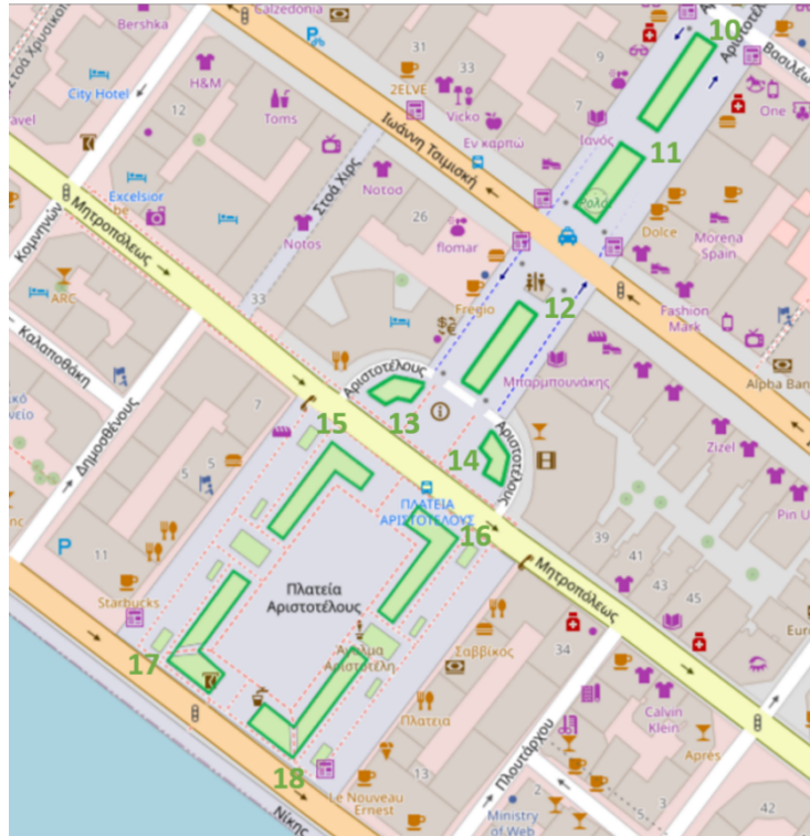
Figure 14: Placement of rain gardens 10–18 within existing landscaped areas along the Aristotelous Square axis (Source: e-poleodomia)
