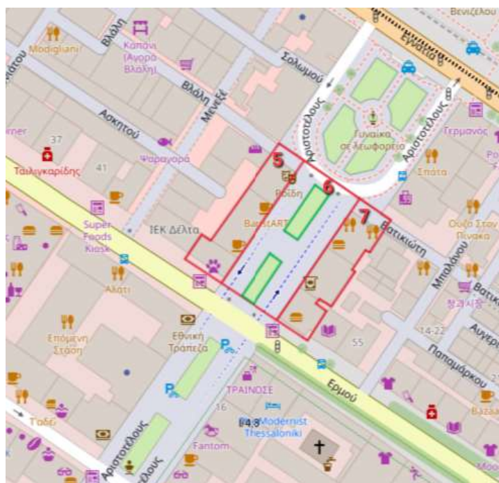
Figure 8: Subdivision of the study area into subcatchments along the Aristotelous Square axis, between Egnatia and Ermou Street (Source: e-poleodomia)
