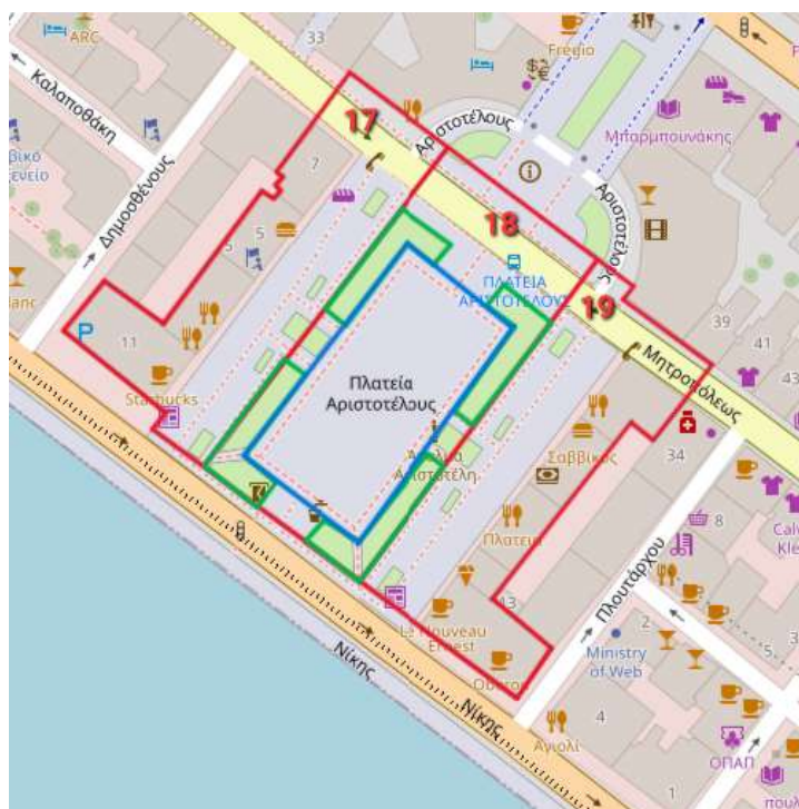
Figure 12: Subdivision of the study area into subcatchments along the Aristotelous Square axis, between Mitropoleos Street and Nikis Avenue (Source: e-poleodomia)
