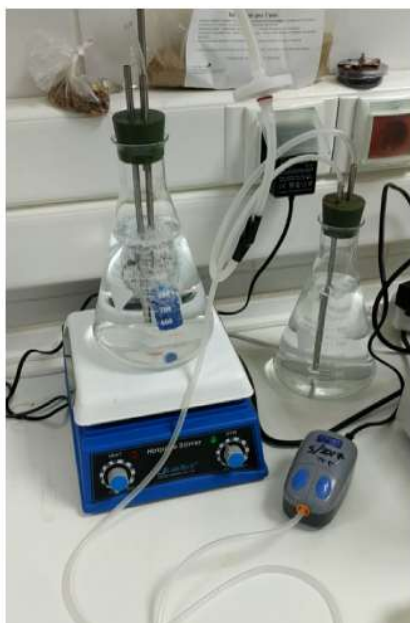
Figure 2. Draw and Fill reactor used
